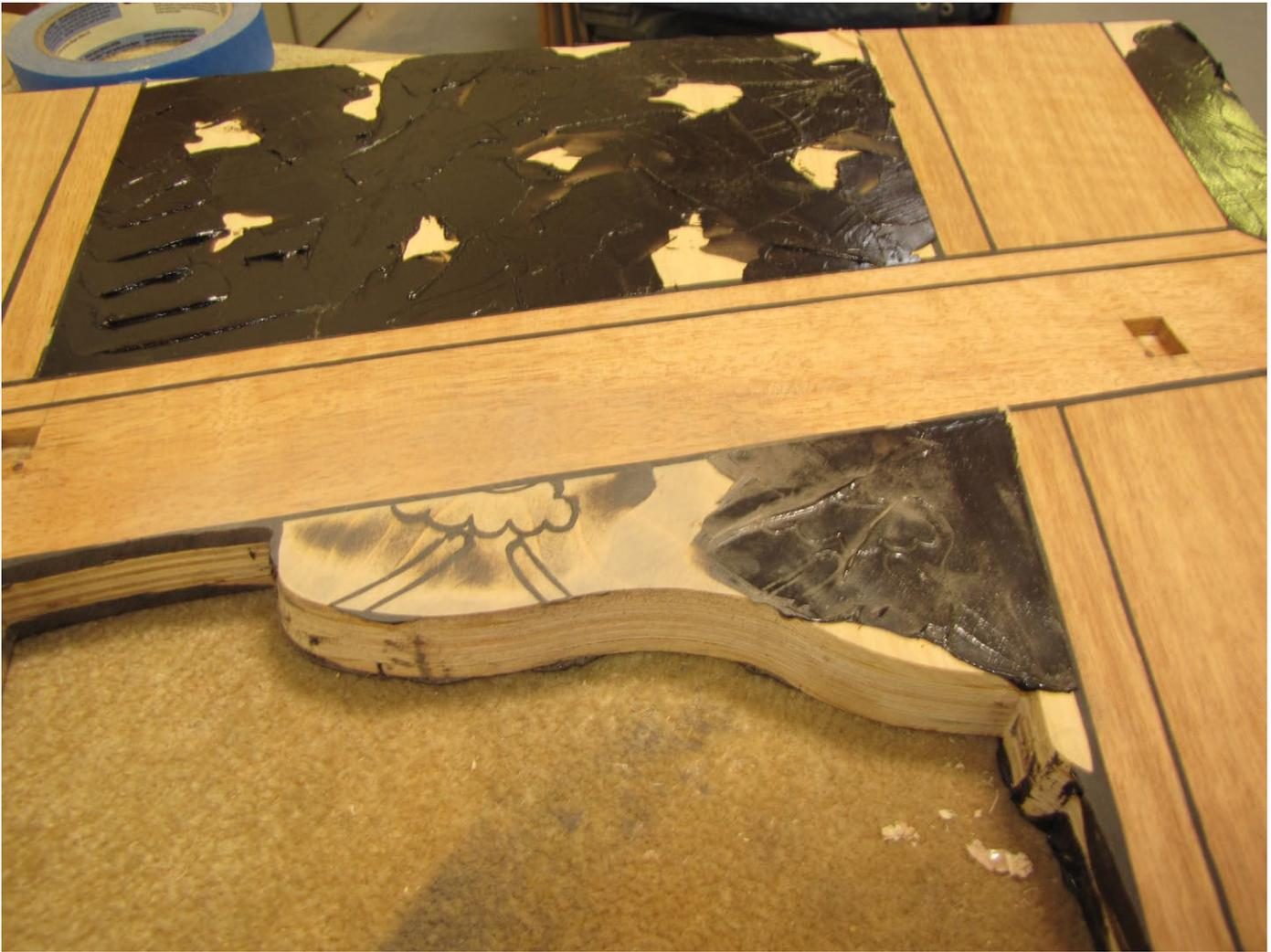
Fig. 4. Detail of epoxy work in progress, Cederquist studio 2013.
