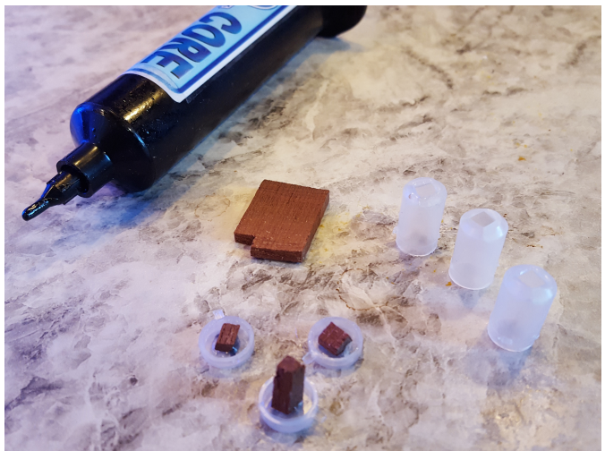
Fig. 3. Embedding wood specimens in plastic capsules with the Tuffleye Core embedding resin.
