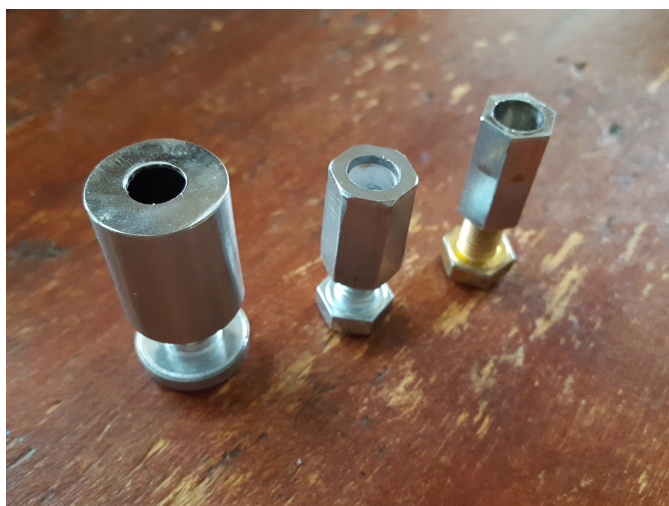
Fig. 4. Different prototypes for a hand microtome, made out of coupling nuts.
